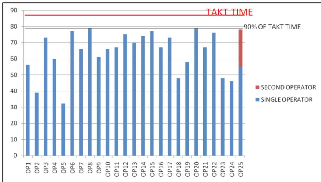
Figure 3: Operator load charts (from operator -1 to operator-25) after KAIZEN
