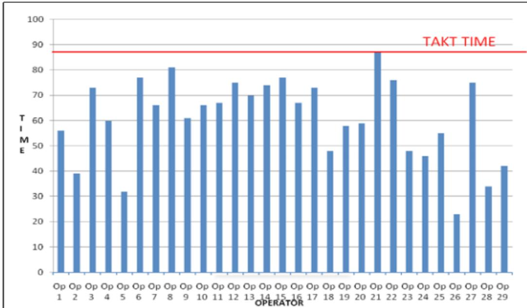
Figure 1: Operator load charts (from operator -1 to operator-29) before KAIZEN
