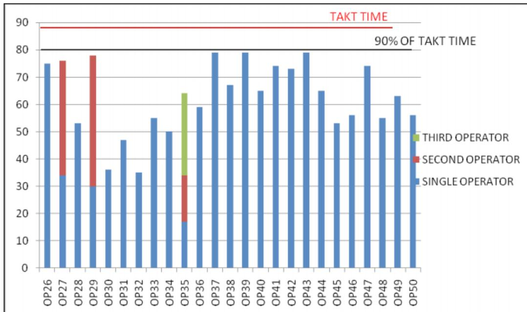
Figure 4: Operator load charts (from operator -26 to operator-50) after KAIZEN
