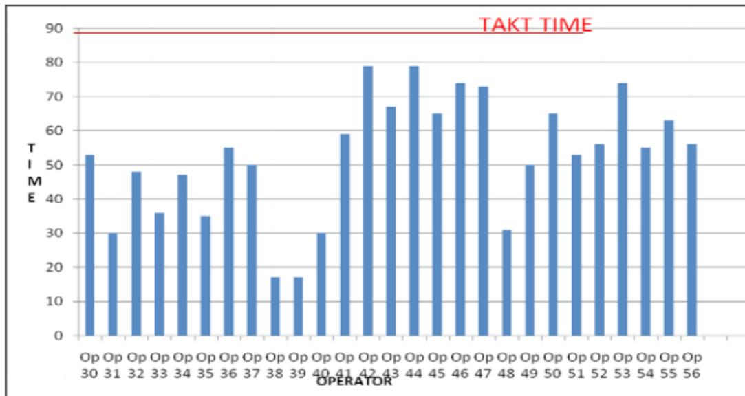
Figure 2: Operator load charts (from operator -30 to operator-56) before KAIZEN
